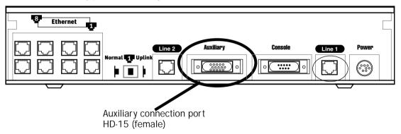
By default, the Auxiliary port on your Netopia R5000 Series is enabled for remote console-based management via an external modem. This means that all you have to do is connect your modem to the Auxiliary port and configure the router for any AT command string your modem requires in the **Line Configuration** screens under the **WAN Configuration** menu.
